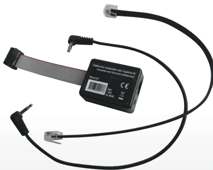
LIP-EHS • Enables the connection of a wireless headset (without the need to use a handset lifter) • Suits iPECS LIP-8012E and LIP-8024E handsets only • Supports wireless headsets from GN Netcom® / Jabra™ and Plantronics® Inc.
